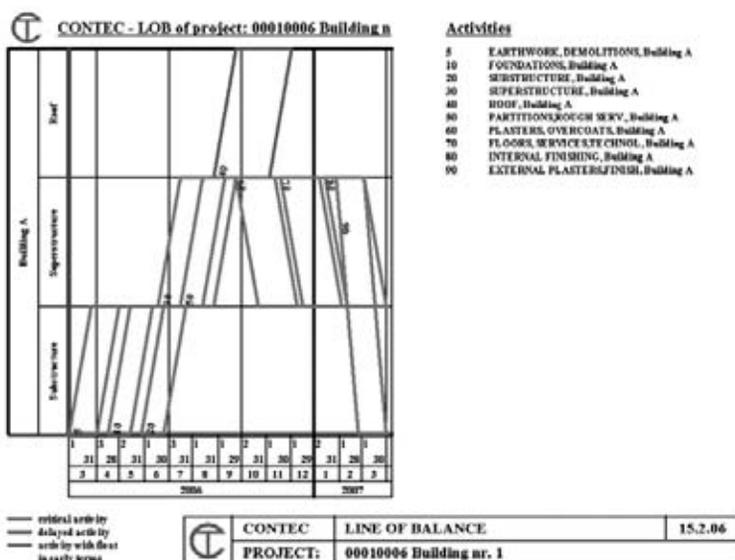
Figure 4. Example of the aggregated simple line-of-balance (time-space graph) into activity
