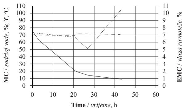
**Figure 3** Moisture content – timber stack weight basis (—), drying temperature (---) and EMC (...) in drying procedure 3
