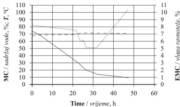
**Figure 2** Moisture content – timber stack weight basis (—), drying temperature (---) and EMC (...) in drying procedure 2
