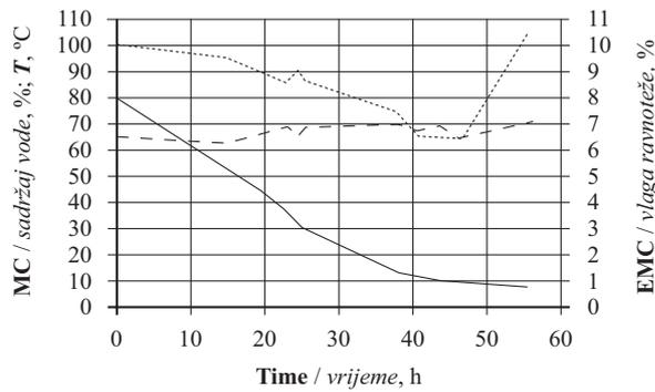
**Figure 1** Moisture content – timber stack weight basis (—), drying temperature (---) and EMC (...) in drying procedure 1
