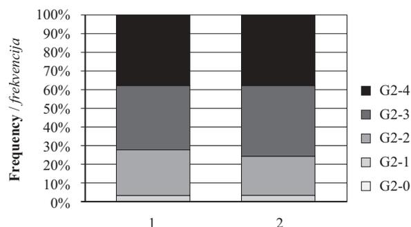
**Figure 6** Frequency distribution of graded spruce sawnwood before (1) and after drying (2) by procedure 1 (G2-0...1<sup>st</sup> class; G2-4...the last class)
