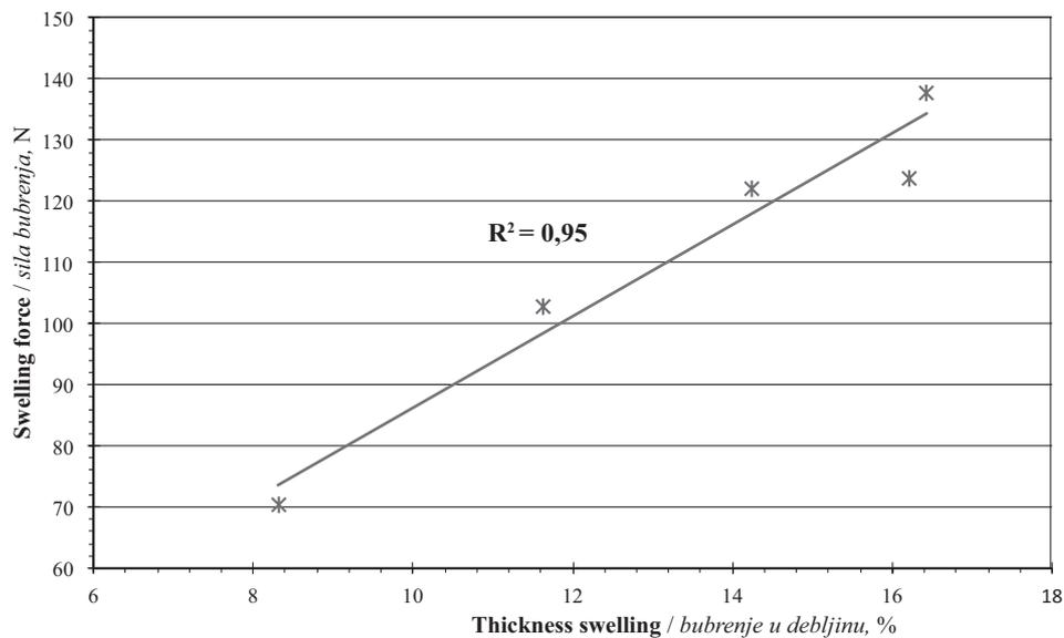
**Figure 4** Correlation between thickness swelling and swelling force
