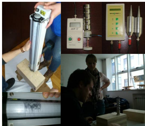
Figure 2 Measurements and devices; resistographic measurements (left) and hygrometric measurements (right)
