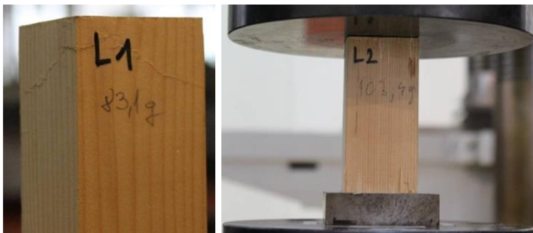
Figure 4 Compression tests after (left) and during (right) destructive testing
