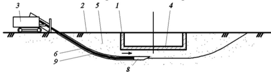
Figure 2 Drawing the injector in the well
