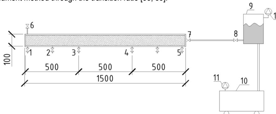
**Figure 5** Scheme of the laboratory test bench for injections 1–8 — taps; 9 — mortar tank; 10 — compressor; and 11 — gauge (dimensions are in millimeters)
