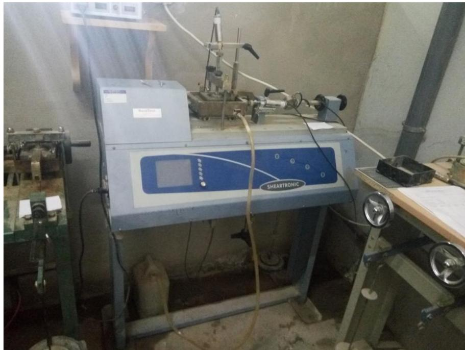
Figure 5 Direct-shear test apparatus
