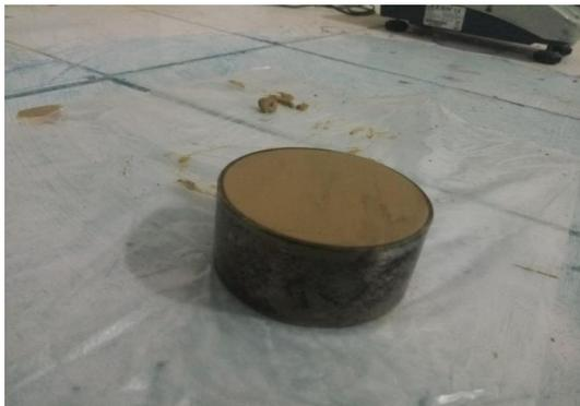
Figure 3 Compacted sample in the mold
