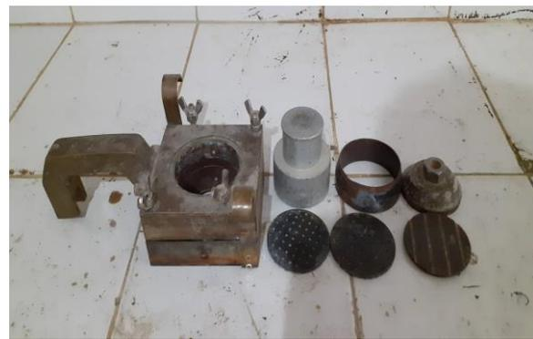
Figure 4 Disassembled shear box
