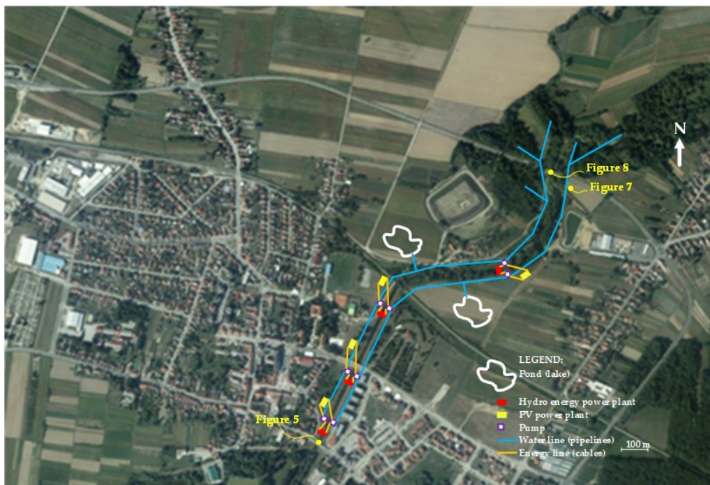
Figure 7. Suggestion of the facilities and objects of the monkey cheek concept of flood prevention
