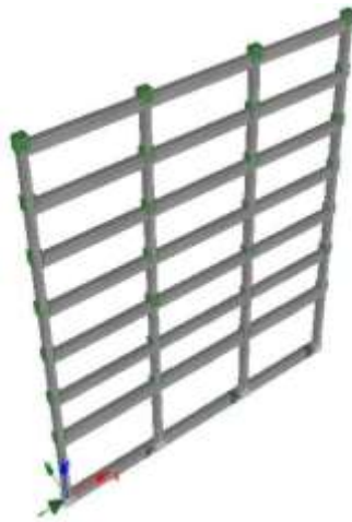
Figure 2. 2D modelling of the studied frame in SeismoStruct
