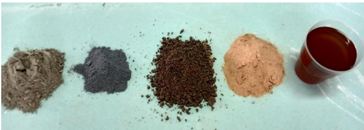
Figure 1. Raw materials used to prepare high-performance sand concrete: (a) ordinary Portland cement, (b) SF, (c) crushed sand, (d) dune sand, and (e) superplasticizer
