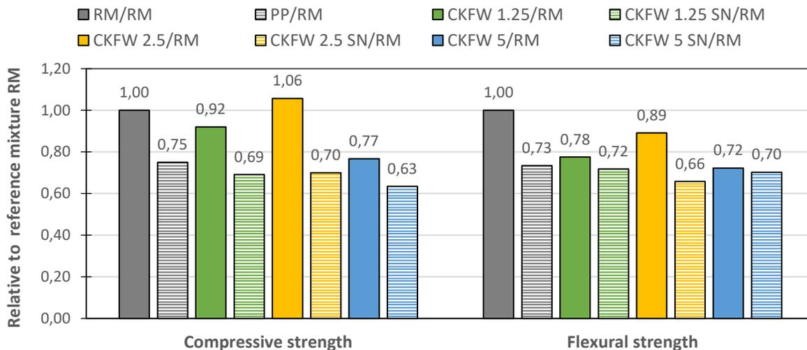
Figure 5. Compressive and flexural strengths relative to the reference mixture RM
