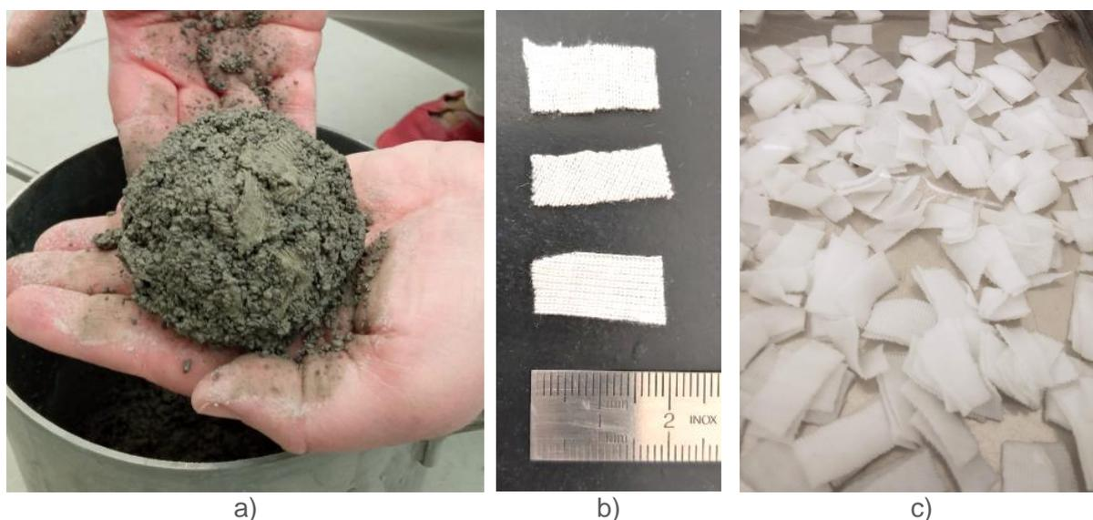
**Figure 2. a) Screed snowball test; b) Pieces of cotton knitted fabric waste (CKFW); c) CKFW saturation in tap water**
