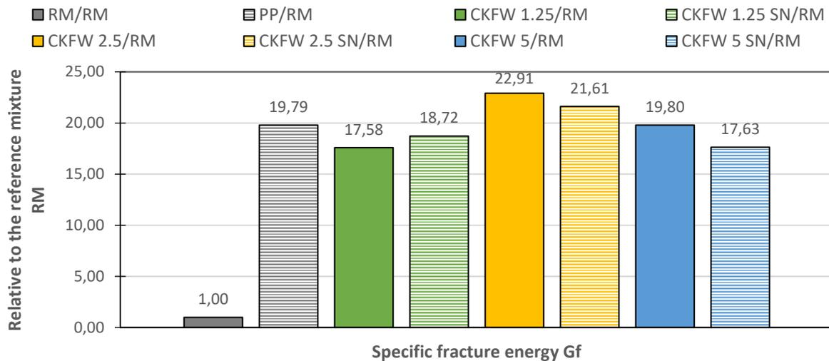
**Figure 9. Specific fracture energy  $G_f$  relative to reference mixture RM**
