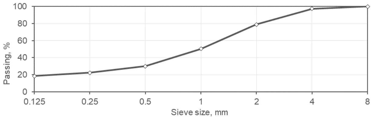
Figure 1. Particle-size distribution of dry ready-mix screed
