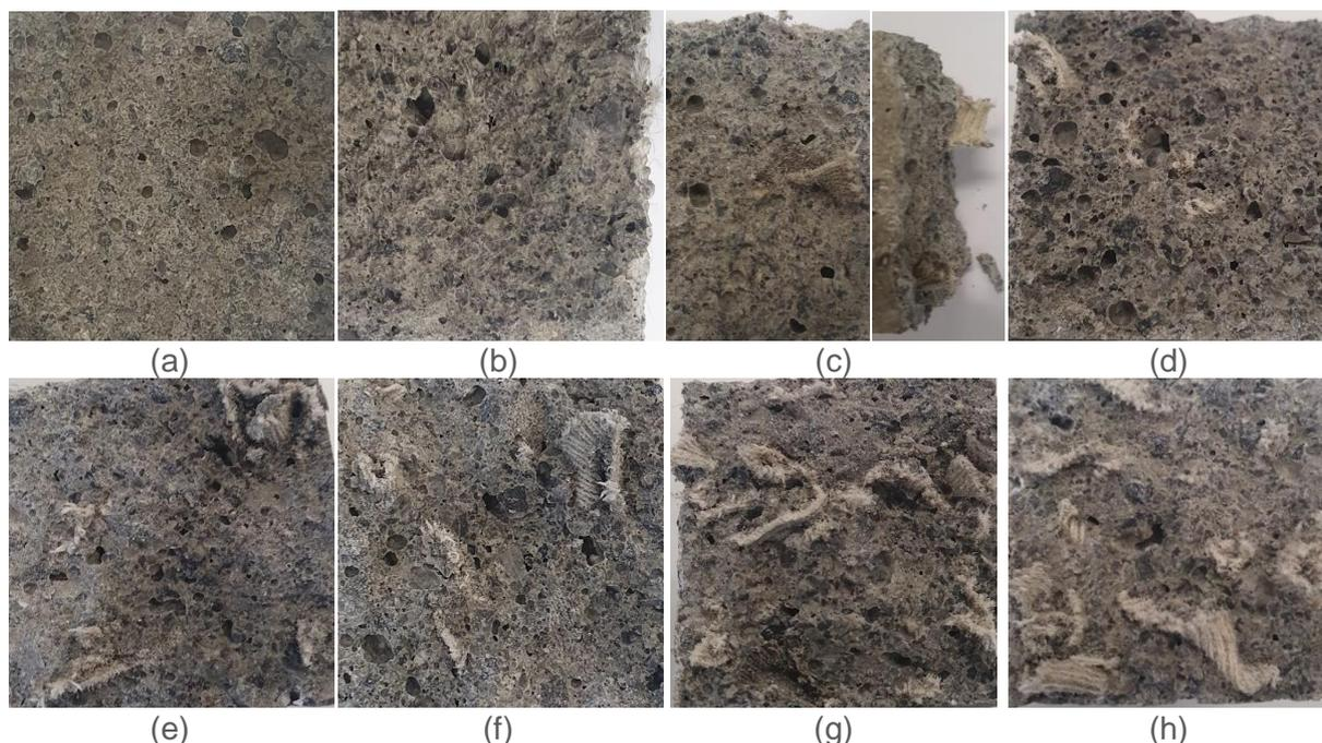
**Figure 7. Screed specimens after fracture: a) RM; b) PP; c) CKFW 1,25; d) CKFW 1,25 SN; e) CKFW 2,50; f) CKFW 2,50 SN; g) CKFW 5,00; h) CKFW 5,00 SN**
