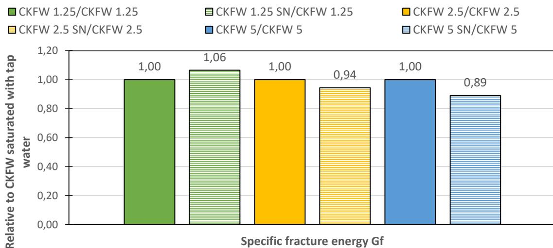
**Figure 10. Specific fracture energy  $G_f$  of CKFW specimens relative to CKFW saturated with tap water specimens**
