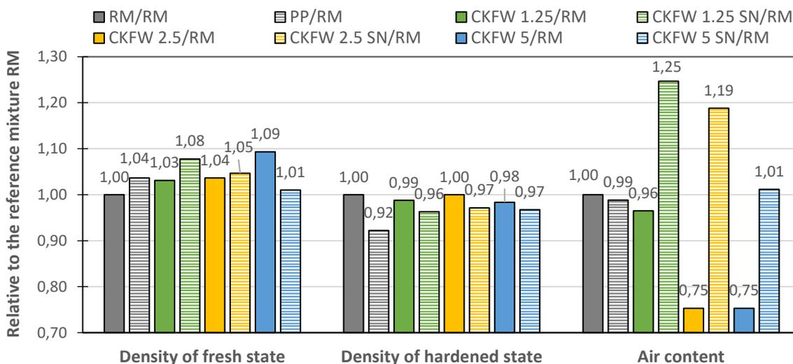
**Figure 4. Densities in fresh and hardened states and air content of screeds relative to the reference mixture RM**
