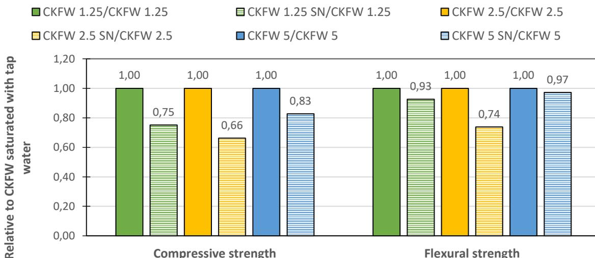
Figure 6. Compressive and flexural strengths of CKFW specimens relative to CKFW saturated with tap water specimens
