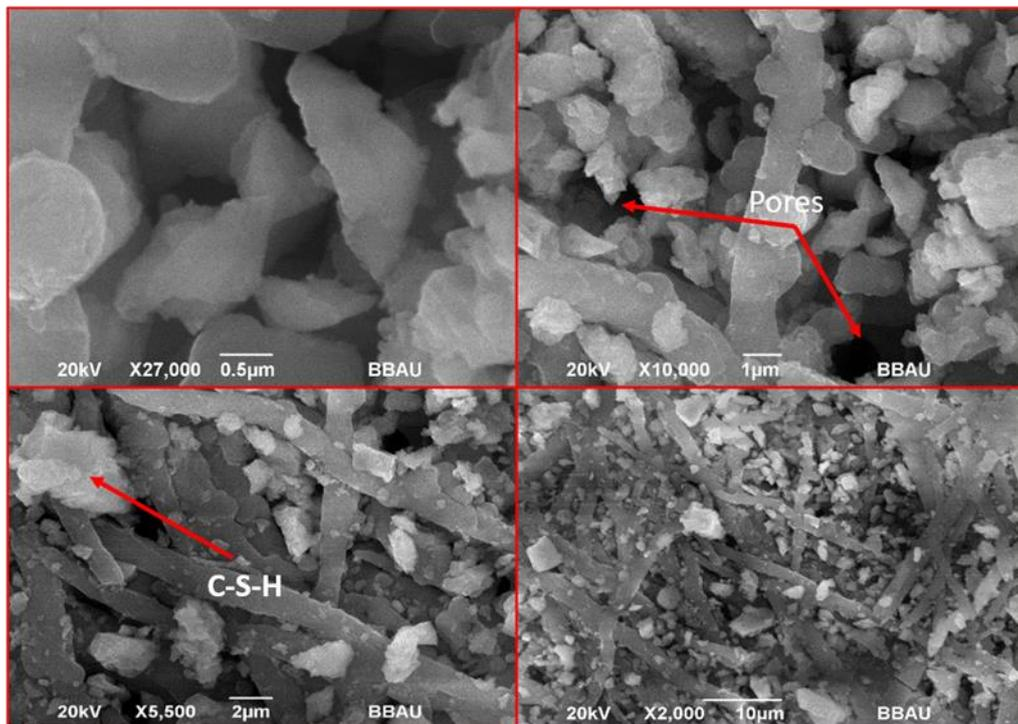
**Figure 2. Scanning electron microscopy (SEM) of Eggshell at different magnifications**
