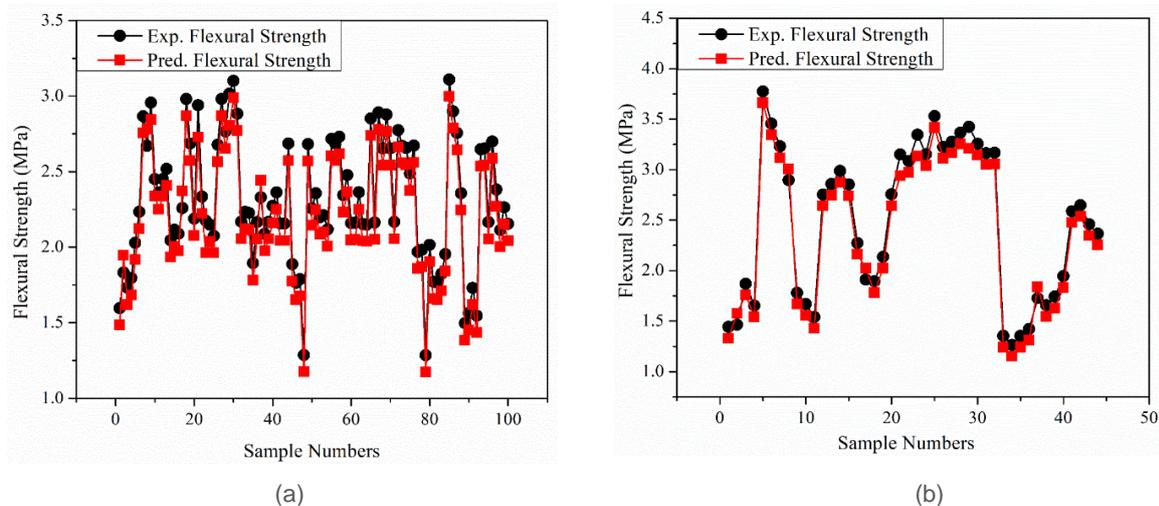
Figure 8. Comparative study of experimental and predicted flexural strength for (a) training and (b) testing
