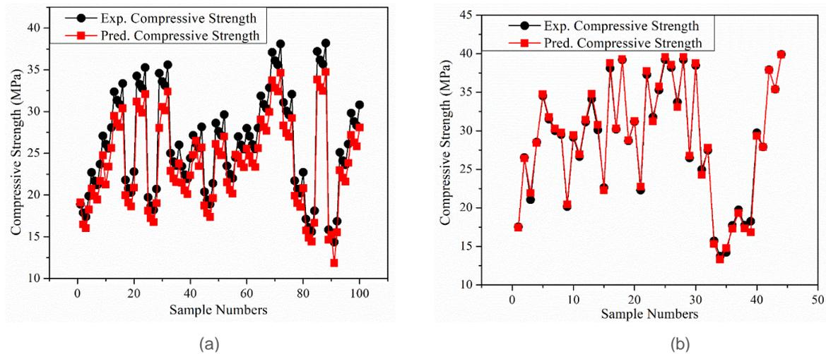
Figure 7. Comparative study of experimental and predicted compressive strength for (a) training and (b) testing
