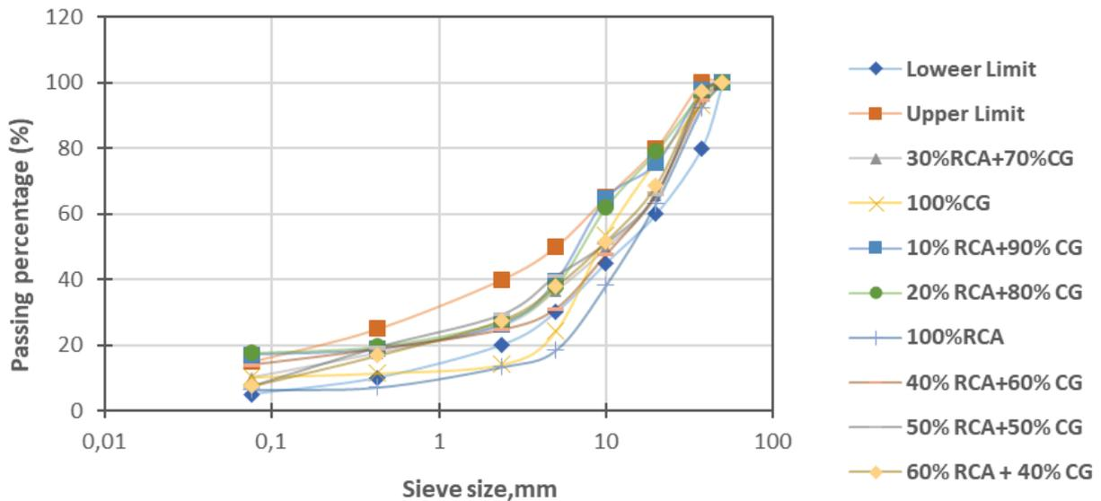
**Figure 3. Particle size distribution of all mixtures used in this study**
