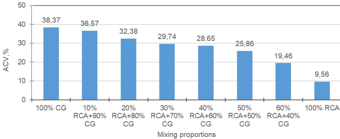
**Figure 4. ACV (%) vs different mix ratio of RCA & CG**
