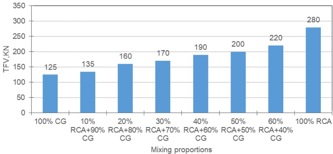
**Figure 5. TFV, kN vs different mix ratio of RCA and CG**
