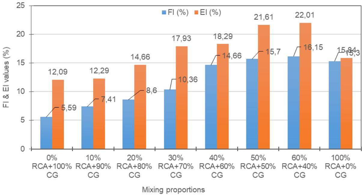
**Figure 10. Graph for flakiness and elongation index of different percentage composition of RCA and CG**
