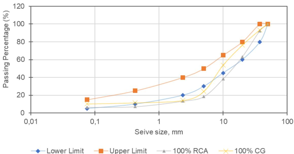
Figure 2. Gradation curve for comparisons of unblended RCA and CG
