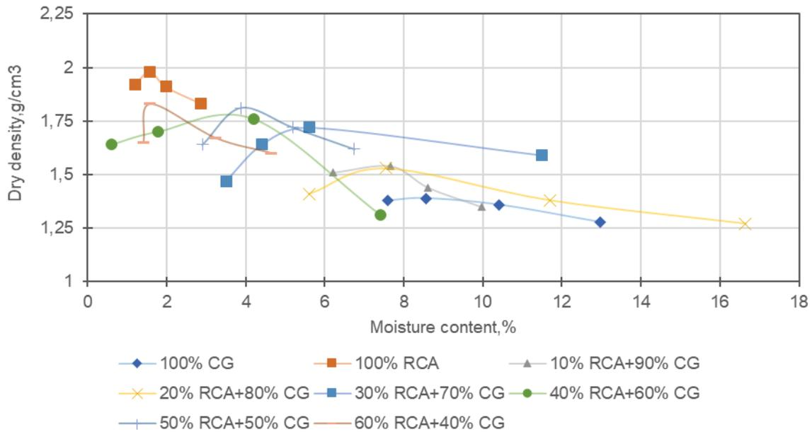
**Figure 8. Moisture-density relation curve of blended RCA and CG**
