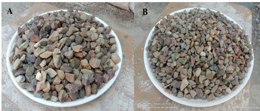
Figure 5. Coarse aggregate utilized in the experiment with different sizes: (a) 20 and (b) 10 mm
