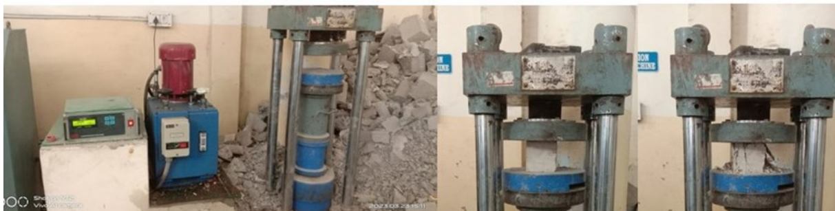
Figure 7. Testing of compressive strength of GPC specimens on 100 mm cubes
