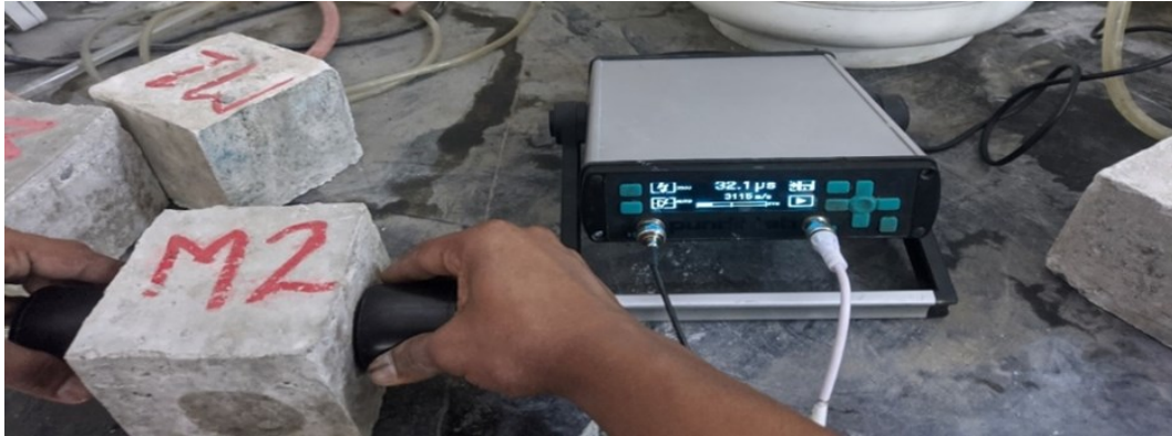
Figure 8. Assessment of ultra-sonic pulse velocity GPC specimens
