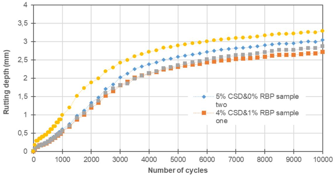
Figure 11. Rutting depth variation with cycles
