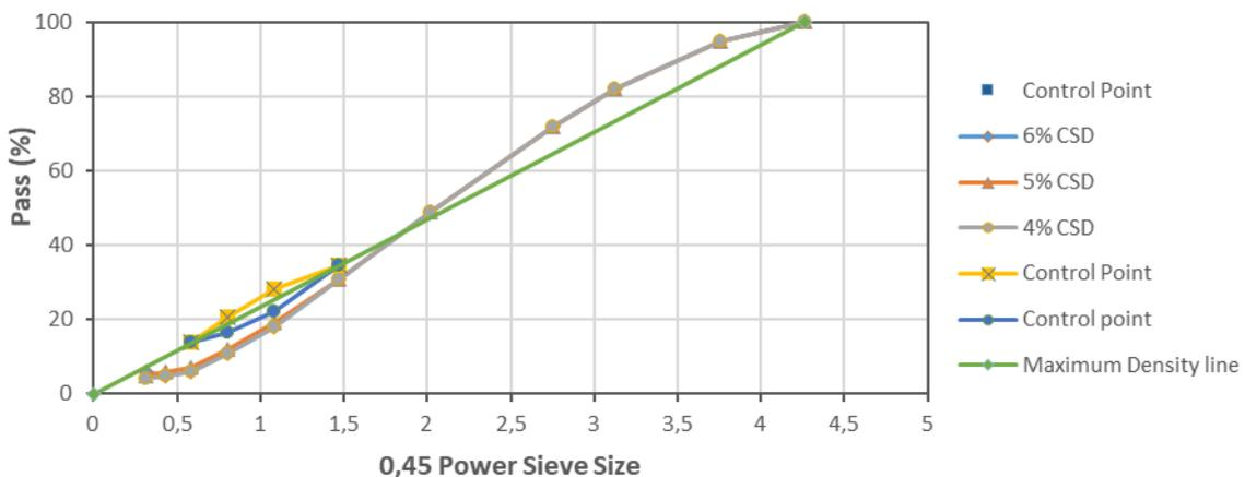
Figure 2. Superpave gradation 0,45 power chart used for 4, 5, and 6 % CSD filler
