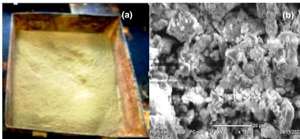
**Figure 3. (a) CSD filler; (b) SEM image of CSD**
