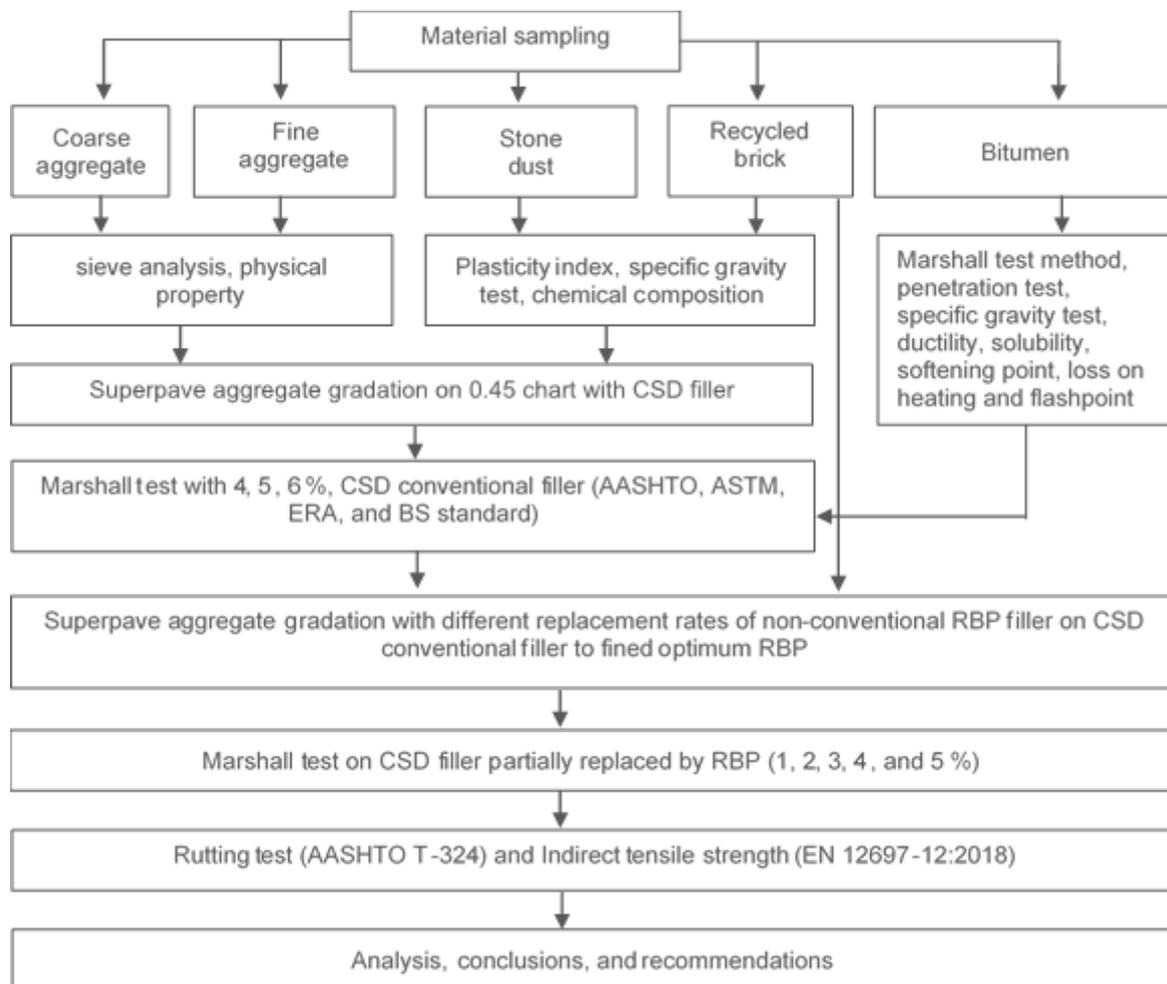
**Figure 1. Overall research approach with 1-5 % recycled brick powder (RBP) replacement**
