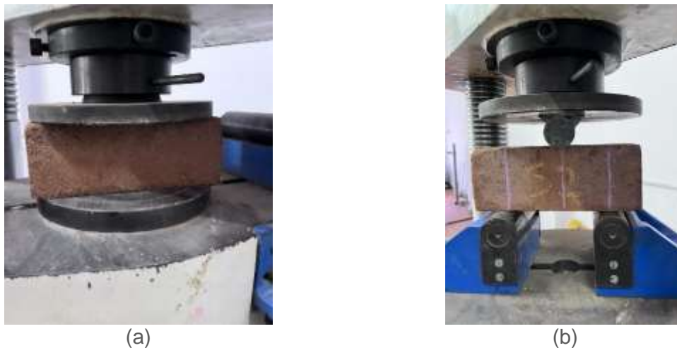
Figure 5. Mechanical test setup: (a) compression test and (b) flexural test
