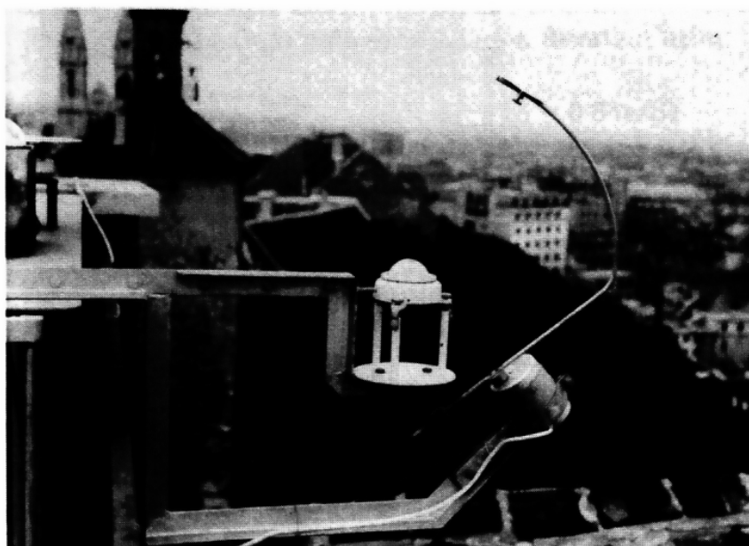
Figure 8. Pyranometer and pyranometer with shadow ring at the central terrace of the Observatory.
