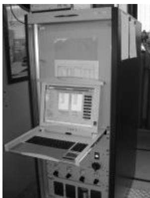
Figure 6: Emission testing system AVL – SESAM 4 (FTIR)
