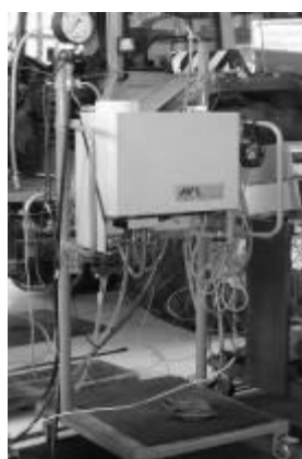
Figure 5: AVL 733S, consumption (regulation in kg·h -1 )
