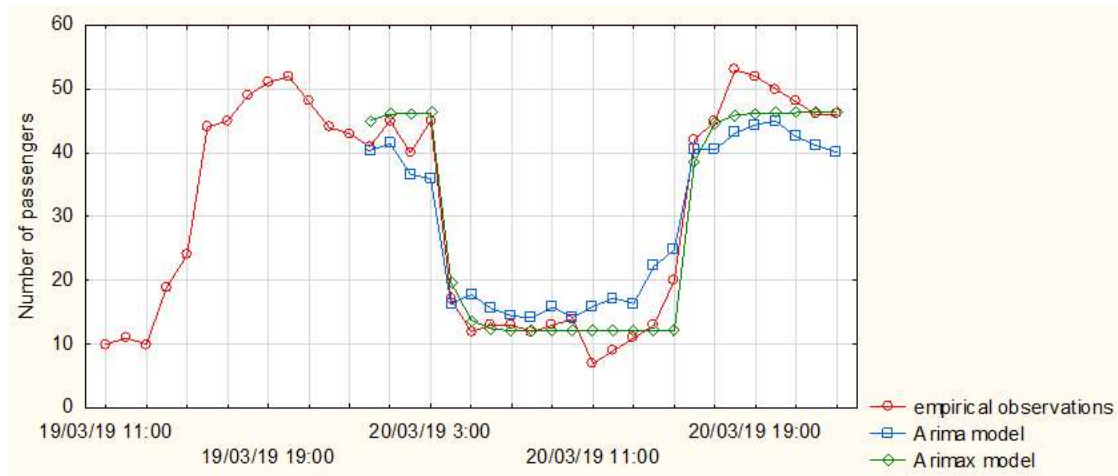
Figure 26. Graph of test observations and forecasts according to the ARIMA and ARIMAX models
