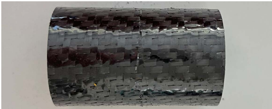
Figure 10 Prepreg material specimen – seawater environment test
