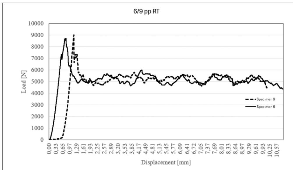
Figure 7 Behaviour of specimens made with prepreg technique and kept at the room temperature
