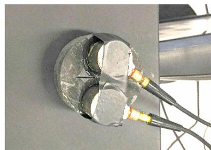
**Figure 2:** Acoustic sensors mounted on the sample on both sides of the Chevron notch.
