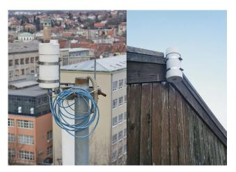
**Figure 1:** Left: The SQM-LE instrument at the RGN site is inside a protective box (white) mounted on the roof of the faculty building. Right: The SQM-LU-DL instrument at the Merenje site is also inside a protective box mounted on the roof of a small shed in the countryside. Both instruments have a clear zenithal area.
