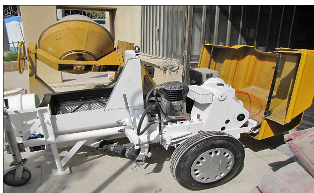
Figure 4: Wet mix shotcreting machine (model T13)
