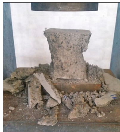
Figure 8: A broken cube sample in a uniaxial compression test
