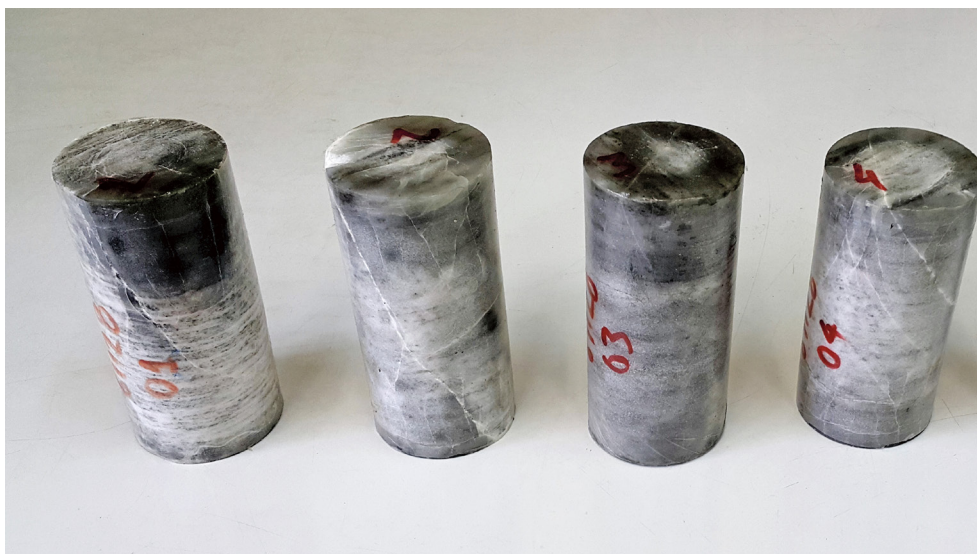
Figure 3: Anhydrite NX specimens used for triaxial tests
