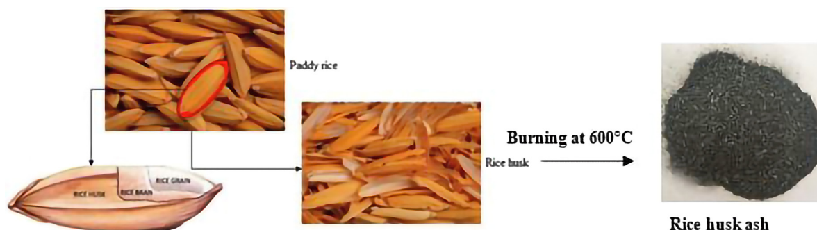
Figure 2: Production of rice husk ash (Derived from Fernandes et al., 2016; Buggenhout et al., 2013; Kieling, 2009).
