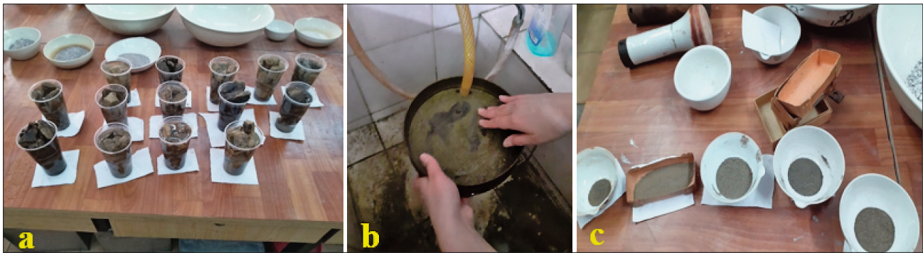
Figure 13: Preparation of samples (a), sample rinsing (b) and dried samples (c).
