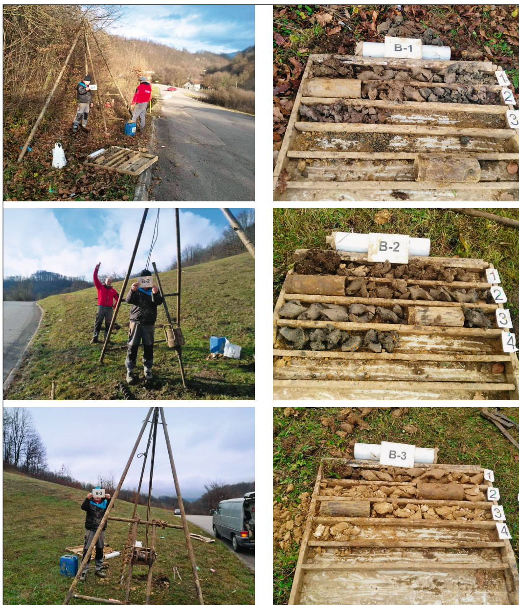
Figure 5: Exploration boreholes B-1, B-2 and B-3
