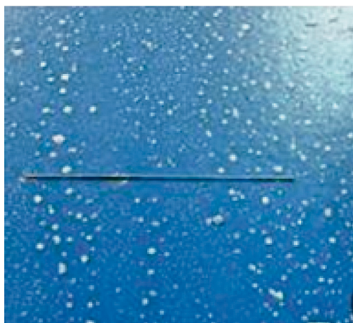
Figure 5: Samples after 240 h of exposure in a salt chamber phosphated sample
