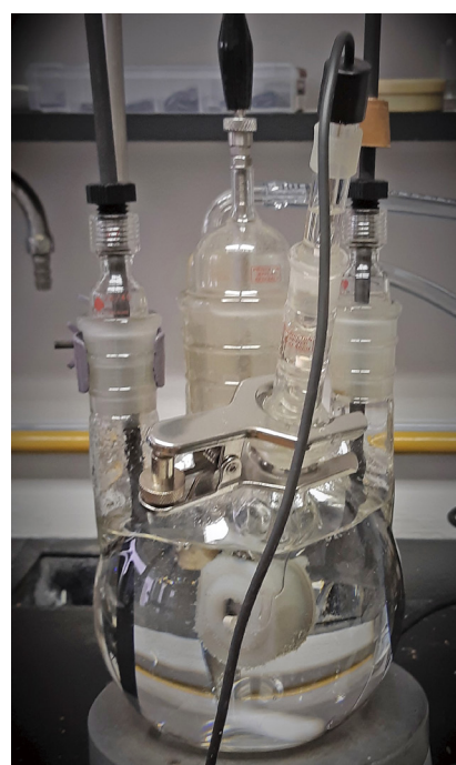
Figure 1: Three electrode corrosion cell
