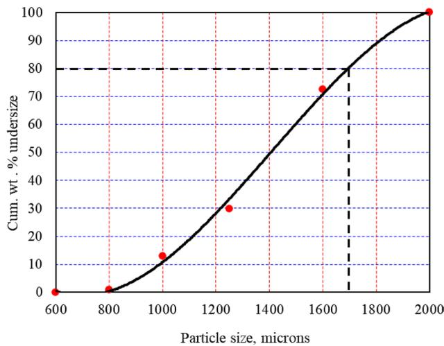
**Figure 2.** Particle size distribution of the head sample
