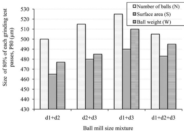
**Figure 3.** The size of 80% of passed ore at various ball loading composition
