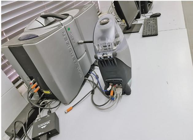
**Figure 1.** Mastersizer 3000 instrument (Yanbu Cement Company Lab, KSA)
