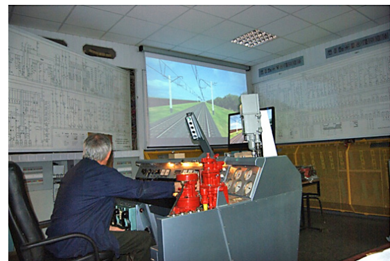
Figure 6: Training simulator for the ChS7 electric locomotive driver
