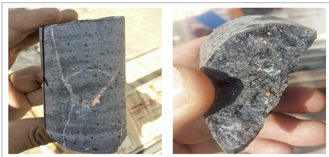
Figure 13: Native copper mineralization in the cores of newly drilled boreholes
