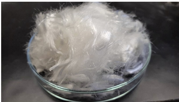
Figure 4: PPFs structure manufactured by the EAMIC company
