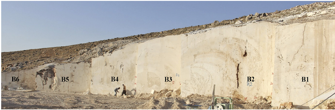
Figure 4: A general view of the Sarchawa marble mining quarry (benches and extraction blocks are shown)
