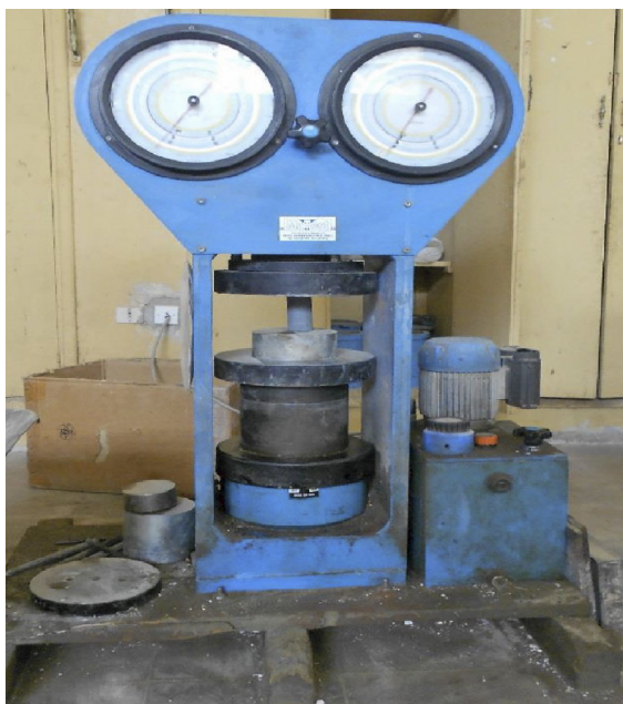
Figure 3: Uniaxial compression test machine
