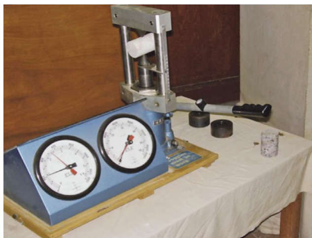
Figure 4: Point load test machine
