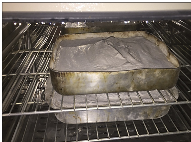
Figure 7: Sample of CKD after soaking prepared for the drying process in an oven
