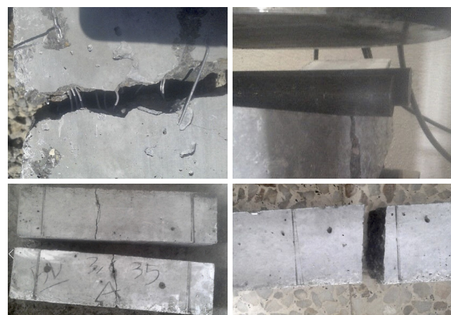
Steel Fiber-Reinforced Concrete Plain Concrete
