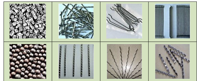
Figure 1: Schematic of steel fibers in different shapes
