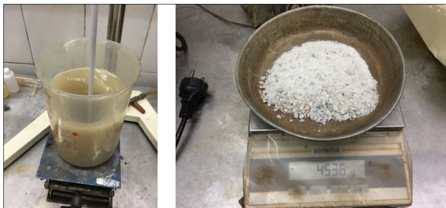
Figure 3: Acid washing process with hydrochloric acid and celestine sample after acid washing process.
