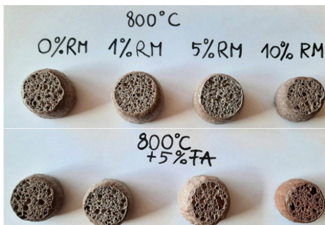
Figure 4: Tablets treated at 800°C with different RM ratios and plus 5 wt % FA
