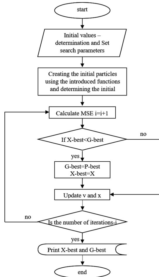
Figure 3: Particle swarm optimization algorithm
