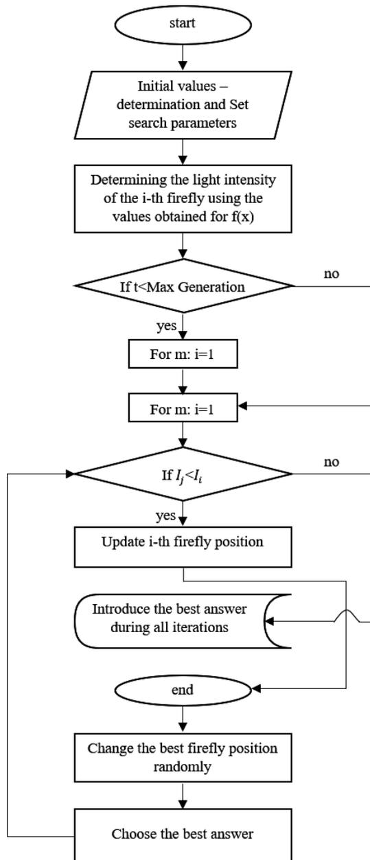
Figure 2: Firefly optimization algorithm
