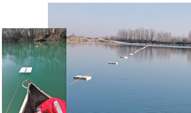
Figure 5: Cable and cable take-outs deployed on the surface
