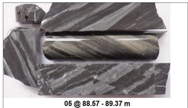
05 @ 88.57 - 89.37 m Figure 5: Cut drill core sample photo of silty tuff with sandy tuff intercalations
