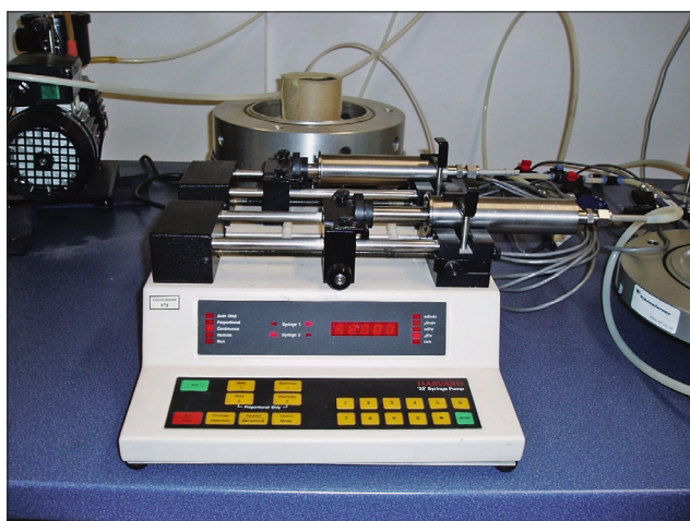
Figure 7: Harvard '33' Syringe Pump
