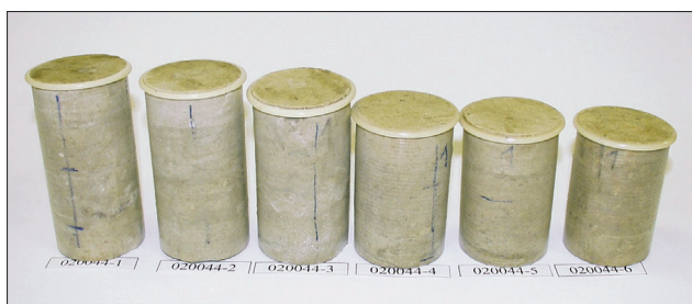
Figure 2: Undisturbed samples of swelling material in the form of a tall cylinder
