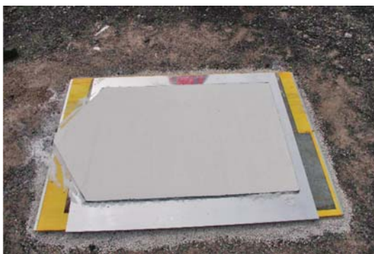
Figure 8: Aluminium sheet casing filled with ground ANFO explosive
