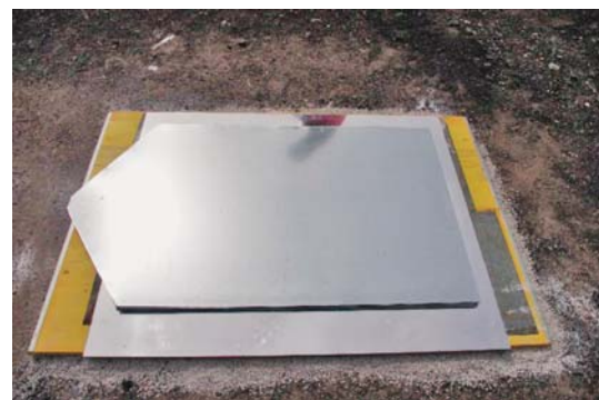
Figure 8: Aluminium sheet casing filled with ground ANFO explosive
