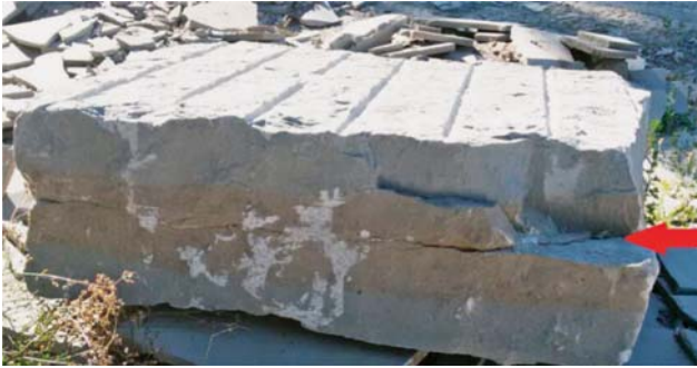
Figure 2: An unfit extracted stone block considered as waste because of a fracture surface indicated on this figure by a red arrow (Elkarmoty et al., 2016)
