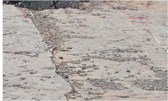
Figure 3: Some outcropping sub-vertical fractures in the bench. The fracture's out-crops are semi-parallel and perpendicular to the bench face.
