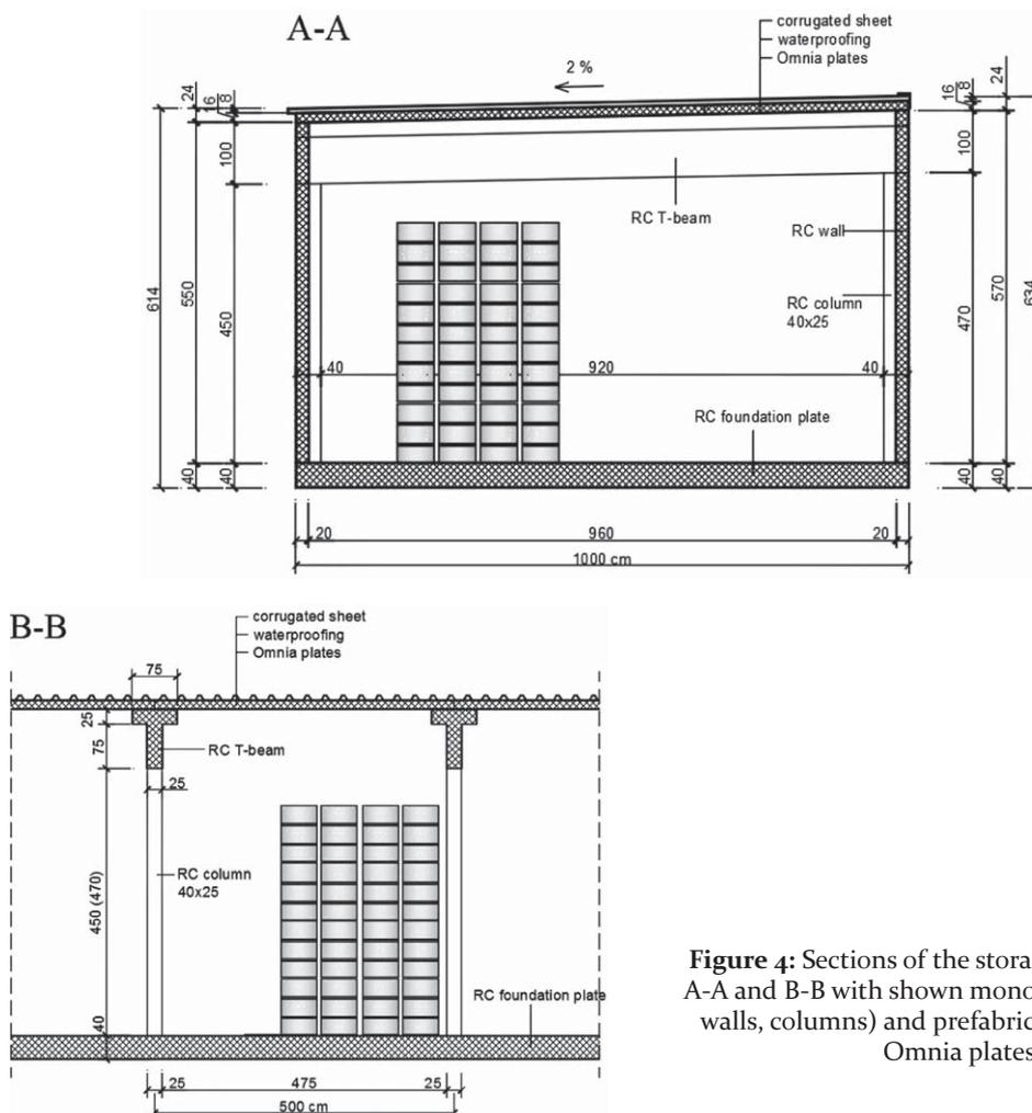
Figure 4: Sections of the storage facility in the profiles A-A and B-B with shown monolithic (foundation plate, walls, columns) and prefabricated (T section beams, Omnia plates) parts
