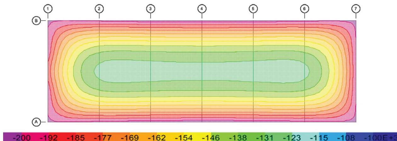
Figure 10: The soil pressures of the base plate for the vertical load for ULS [kN/m<sup>2</sup>]
