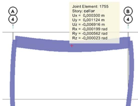
**Figure 8:** Displacements during the earthquake load for SLSE
