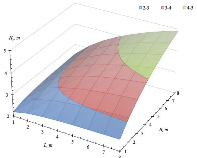
**Figure 10:** The dependence of rational ledge height from the monolith blocks size for category II ( $V_{bl} > 3$  m<sup>3</sup>) at  $n = 0,47$
