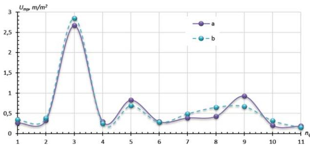
**Figure 6:** The result comparison of specific fracture determination  $U_{mp}$  immediate and remote measurements for the appropriate photos number  $n_{\phi}$  (where  $a$  – direct measurements,  $b$  – remote measurements)
