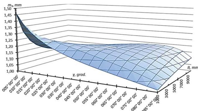
Figure 1: The dependence of the accuracy the spatial coordinates  $m_y$  from convergence angle  $\gamma$  and the basis  $B$  in the case of convergent surveying
