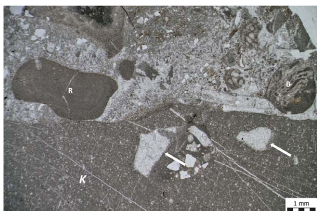
Figure 13: Photomicrograph of conglomerates with a large angular fragment of pelagic limestone in the lower part possibly of the Cretaceous age (K), with geopetally filled Gastrochaenolites boring traces (original upward position marked by arrows), rhodoliths (R) and bryozoans, some of which grew inside the date mussel burrow (B). Position of thin section is marked by white rectangle in Figure 12 . Thin section MB 1 , Stop T5.
