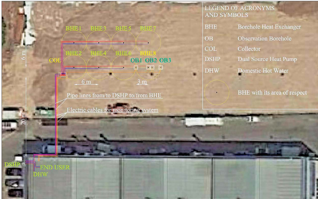
Figure 2: Map of geothermal demo site of Tribano. Therm Arrays of monitoring system are located in OB 1, OB 2 and OB 3 (blue). PT100 are located on the head of BHE 8 and COL (yellow).
