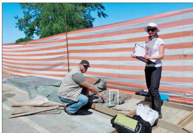
Figure 2: Detailed borehole core determination and in situ measurement of thermal properties in Čakovec. Needle probe inserted into the core is emphasized by a white rectangle.
