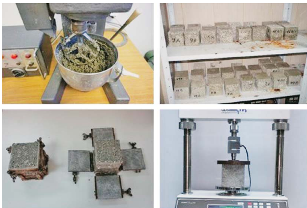
Figure 3: Preparation of concrete mixture, preparation and curing of concrete cubes, and compressive strength testing
