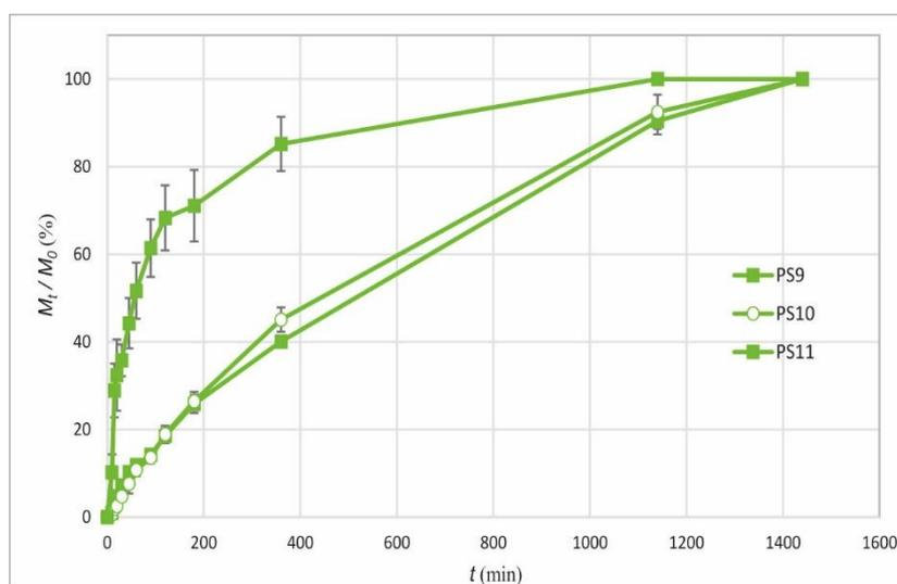
Figure 10. Dissolution profiles for different atomization air flowrate at same polymer content
