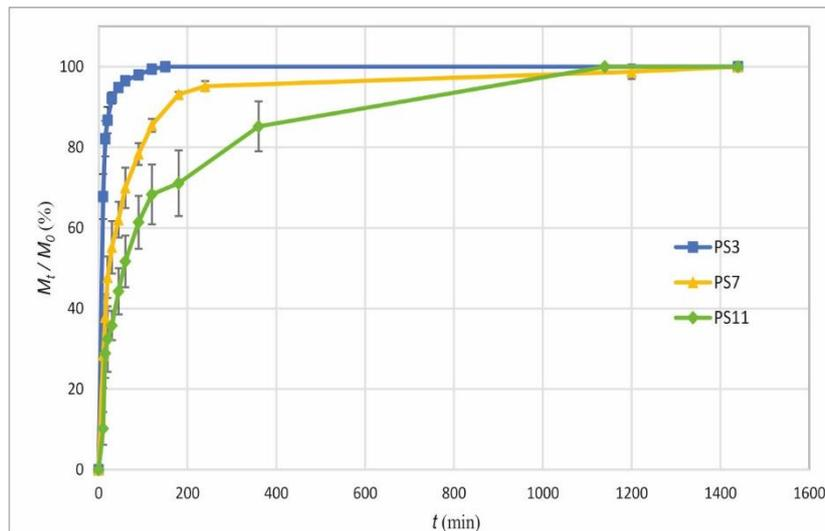
Figure 7. Dissolution profiles for different polymer content at atomization air flowrate  $1.85 \times 10^{-4} \text{ m}^3 \text{ s}^{-1}$
