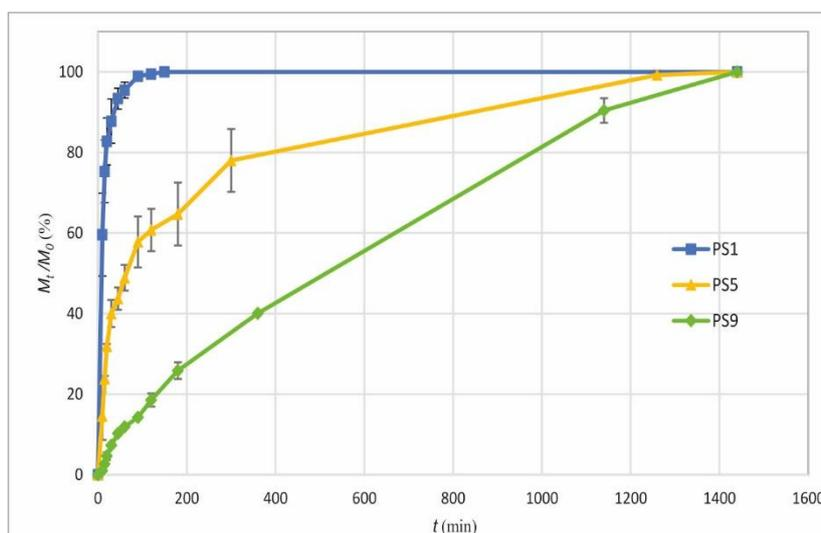
Figure 5. Dissolution profiles for different polymer content at atomization air flowrate  $4.84 \times 10^{-4} \text{ m}^3 \text{ s}^{-1}$
