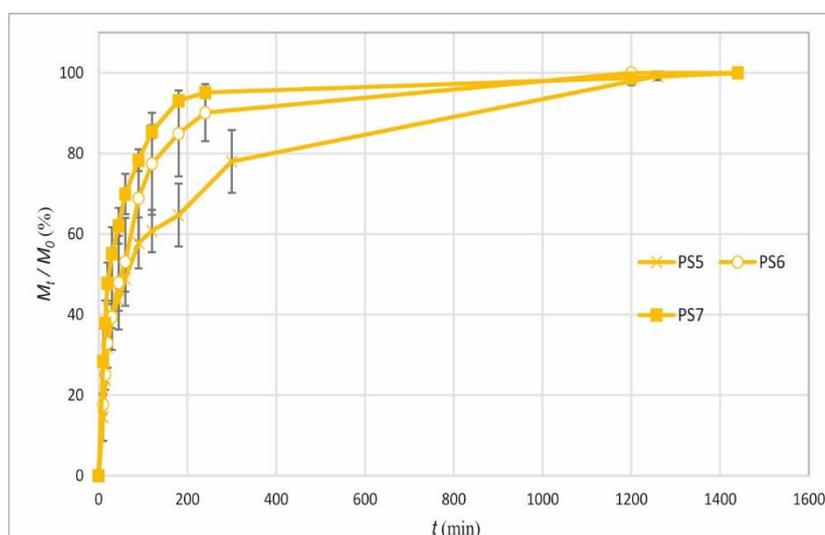
Figure 9. Dissolution profiles for different atomization air flowrate at same polymer content
